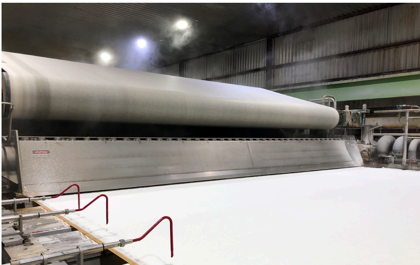
SSV in operation on a pulp machine without any visible steam spillage
